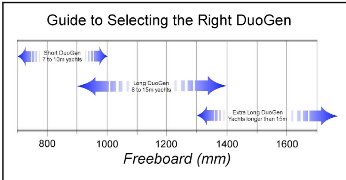
Other factors can also affect tower length choice. For example, where a 38 foot yacht is fitted with a stern arch, the extra-long DuoGen may be preferred to the long because it provides greater clearance above the arch for the air rotor. Equally, a 55 foot yacht that only wished to use the DuoGen in water mode could fit the short tower machine, and simply mount it lower on the transom.
